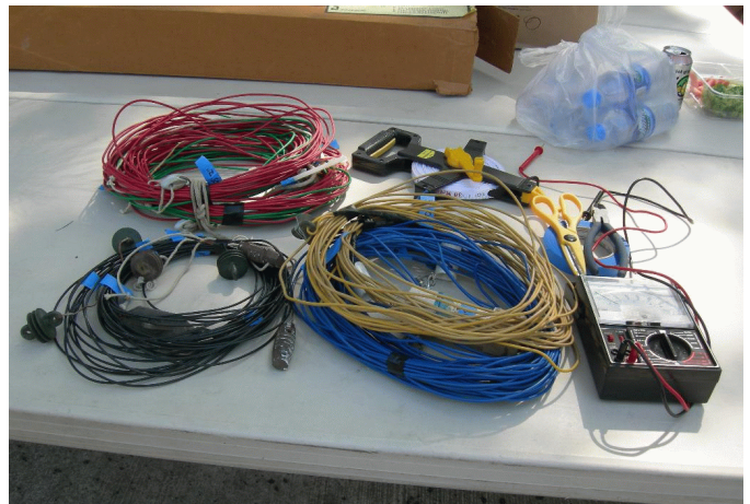
Several wire antennas tested and adjusted as needed
